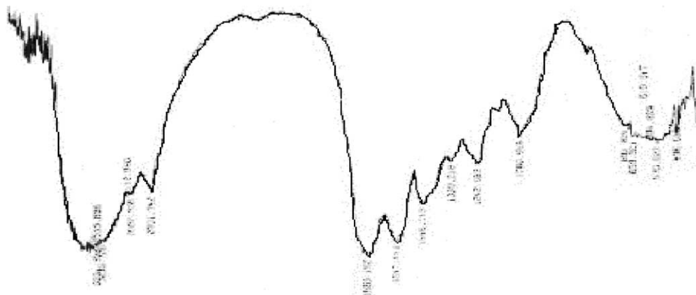
Fig. 4. Fourier transform infrared spectrum of pepsin-soluble bullfrog skin collagen. (The unit of abscissa is \text{cm}^{-1} ).
